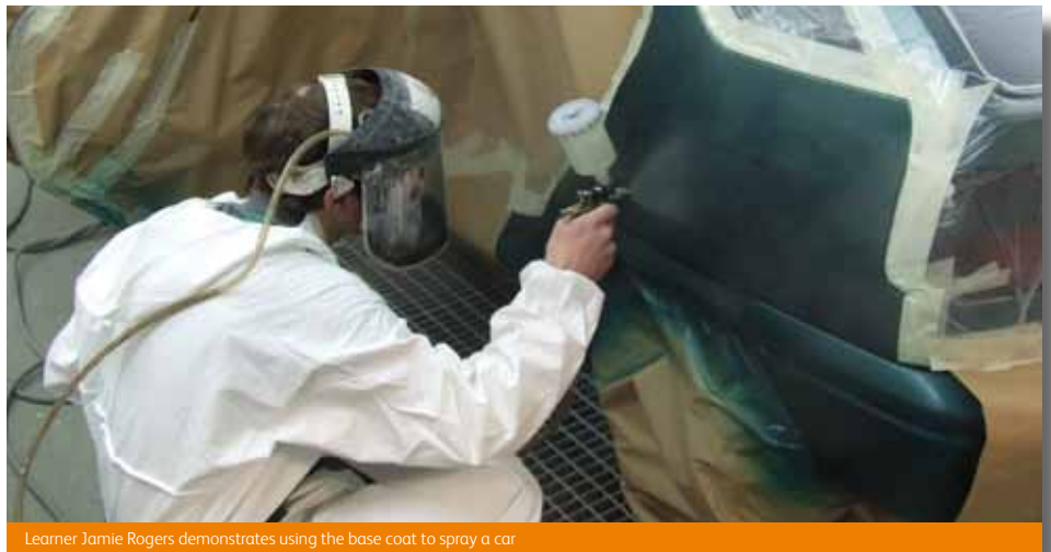
Learner Jamie Rogers demonstrates using the base coat to spray a car
